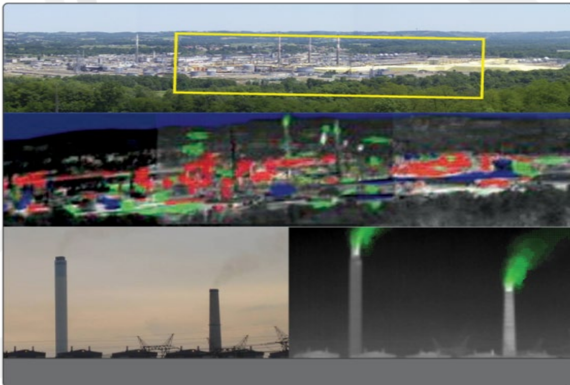
GasViewer Infrared Hyperspectral Imaging Cameras for gas remote detection
