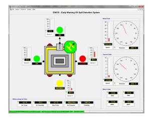
Typical example of combined EWOS and EMS display. Wind, wave and current information can be obtained at a glance.
