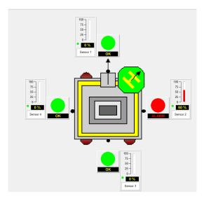
Logic user display can help operators making quick decisions in critical oil spill situations. Alarm levels for each alarm can be adjusted in order to avoid false alarms.
